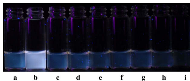
Figure 5. Fluorescence responses of 1 ( 10\ \mu\text{M} ) in the presence of 10 equiv of different anions. (a) only 1 , (b) \text{CN}^- , (c) \text{F}^- , (d) \text{Cl}^- , (e) \text{Br}^- , (f) \text{I}^- , (g) \text{N}_3^- , (h) \text{H}_2\text{PO}_4^- , (i) \text{HSO}_4^- (tetrabutylammonium salt).
